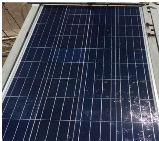
Figure 6.22 Front Surface Cooling by water
