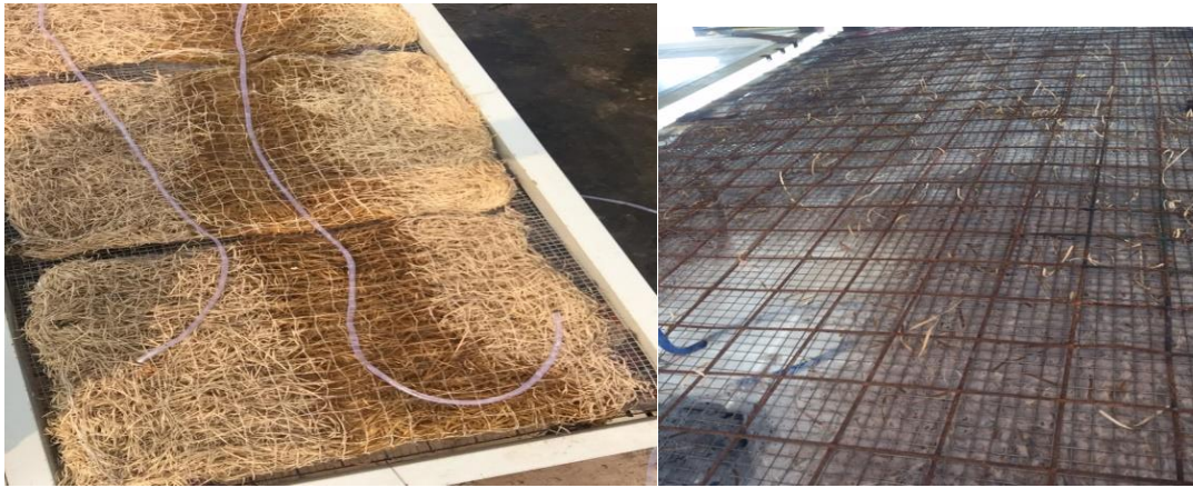
Figure 5.21 Front & Back View of Back Surface Cooling by Common Grass And Water
