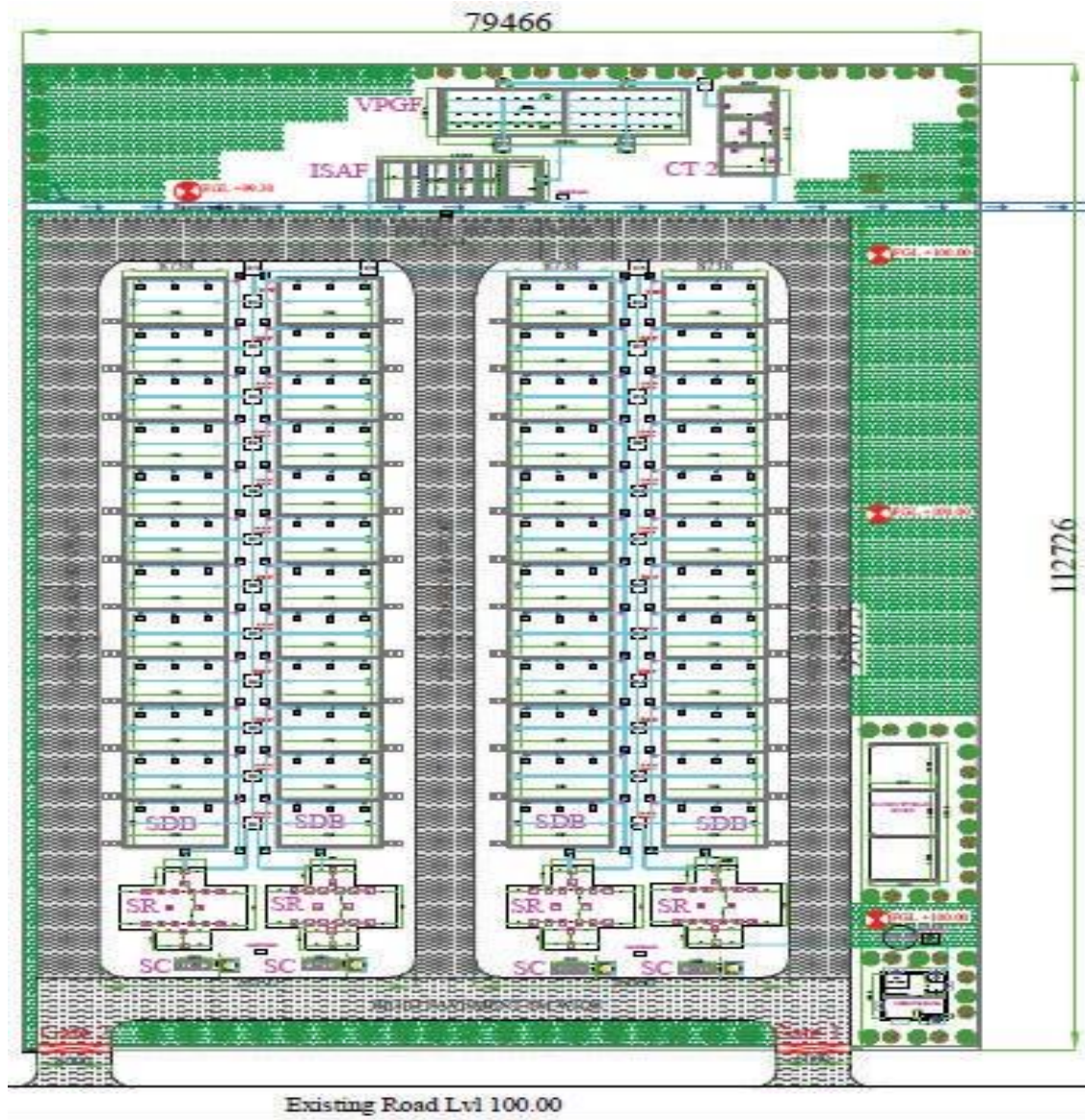
Chart 3.1 Layout of FSTP of 1 Unit of 32 KLD Capacity
