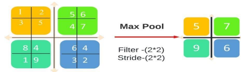
Figure 5.3 Max Pooling operation
