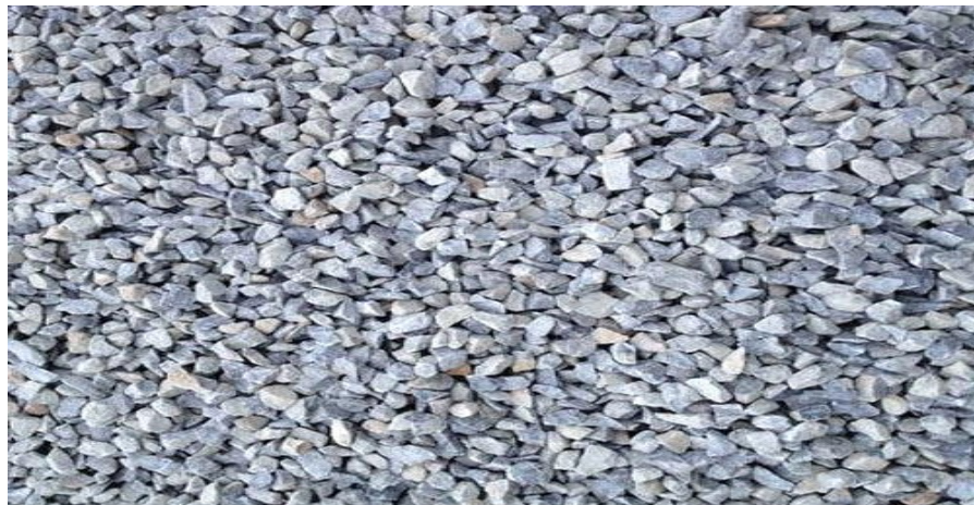
Figure 3.5: Coarse aggregate of 10mm size
