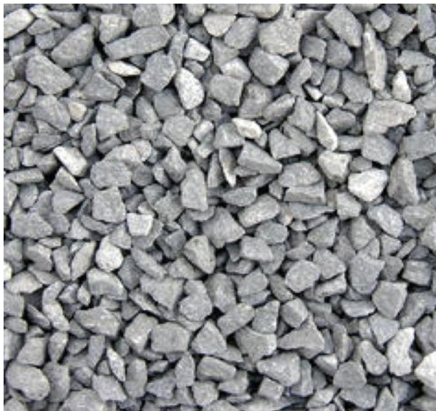
Figure 3.4: Coarse aggregate of 20 mm size
